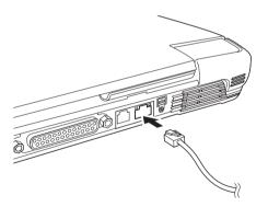
Figure 4-13 Connecting the LAN cable
